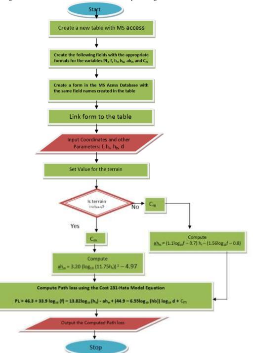
Figure 1 shows the Flowchart for Path loss Analysis using Cost 231-Hata Model
